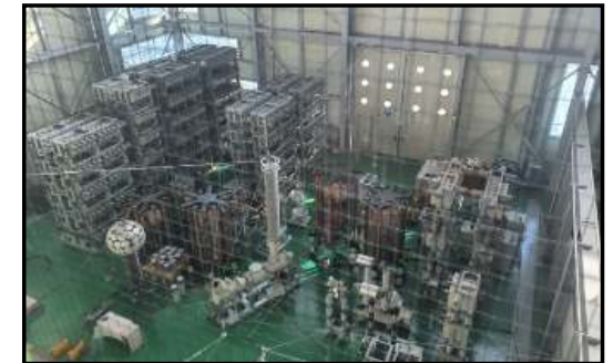
[SLF test using simplified synthetic test in Hyosung]
