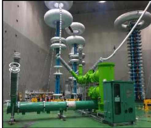
[GIS Dielectric test]
