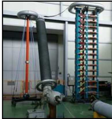
[Dielectric test of Novec mixture gas pressure, mix ratio and shape of poles]
