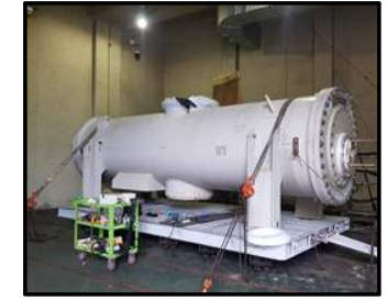
[Internal arc test]
