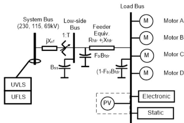
**Figure 2: Comparison WECC Dynamic Composite Load Model (CMPLDW)**
