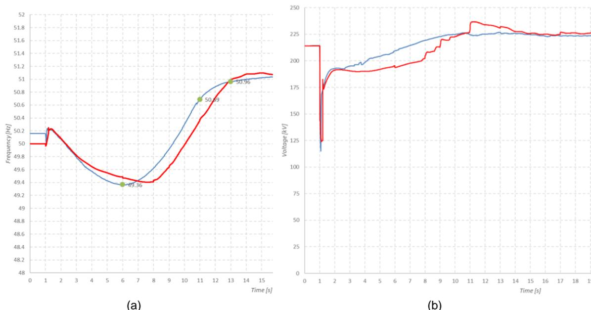
**Figure 3: Frequency (a) and voltage (b) trends around the faulty substation – Real measurements (blue) and simulated (red)**
