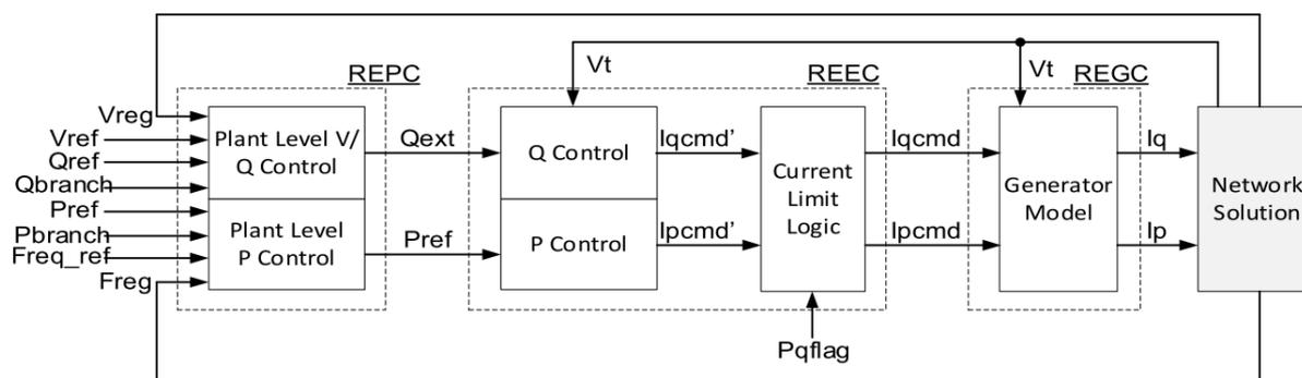
Figure 4: Block Diagrams of Different Modules of the WECC Generic Models (source [13])
