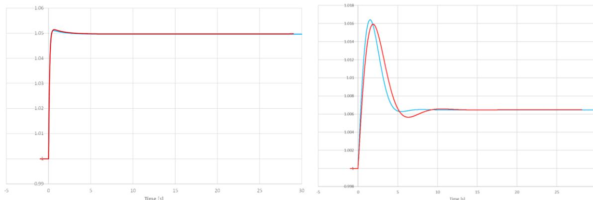
**Figure 1: Comparison between NEPLAN model response (red color) and reference recordings (blue color) for standard tests on Automatic Voltage Regulators and Governors**
