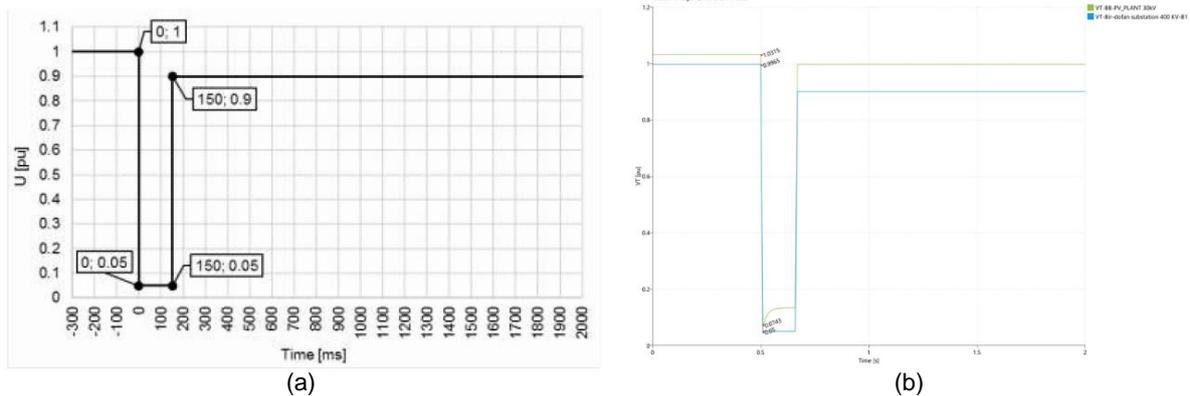
Figure 5: LVRT V-t profile (a) as per GECOL Grid Code [14], and tests results (b)
