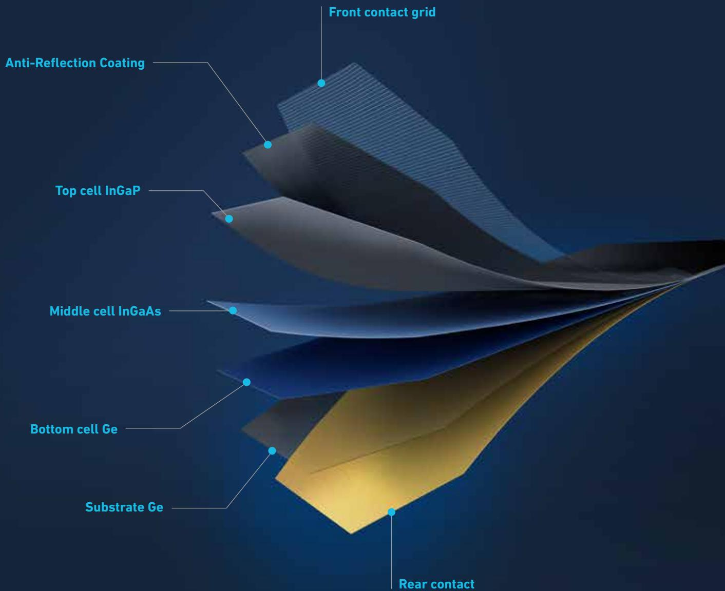
**CESI has more than 30 years' experience in the research, development, and production of high-efficiency space solar cells for civil applications and is one of the top global suppliers of multijunction cells based on III-V semiconductors.**
